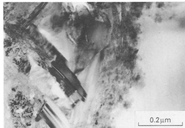
Figure 4 Interphase of 18% V_f sample showing silicon and Al_4C_3 plate-like crystals.
